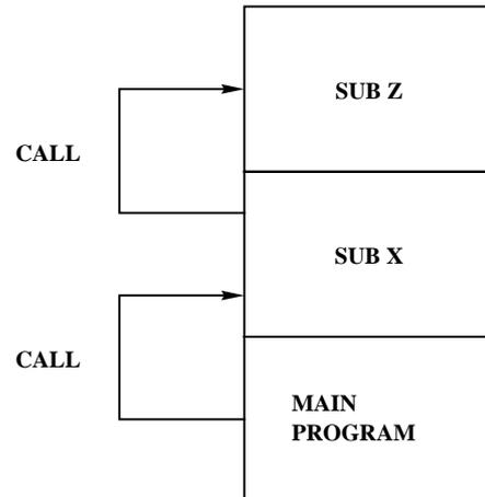
This program is a good example of how *not* to program with ON-condition statements. When subprogram X is called, the ON INPUT # statement is executed. The interrupt is defined in subprogram X and in subprogram Z. When both X and Z are exited, however, the interrupt is no longer defined.
